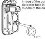
B. Adjust the upper and lower angle adjustment screws and the horizontal adjustment wheel. At this time, the received signal strength is gradually increased. When the signal strength is less than 1.8, please continue to adjust the optical axis.
