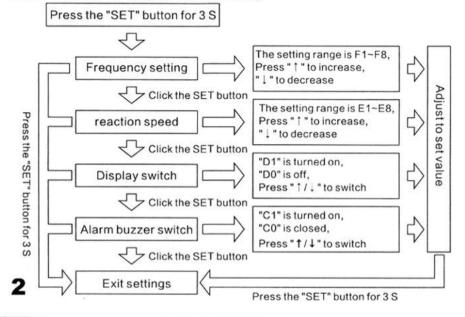
• Response speed setting: the speed when the detected object passes between the transmitter and the receiver to block light. Generally, the speed should be less than the speed required by the intruder to pass through the warning surface. It can be set to 8 gears (E1 ~E8) Alarm response speed (shading time), the smaller the number of gears, the faster the response speed. The shading time is 40ms~180ms, please refer to the following figure for adjusting the shading time.
